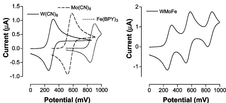
**Figure 6** Cyclic voltammograms of transition metal redox complexes separately (left) and mixed together (right).
