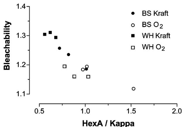
**Figure 2** Bleachability [(unbleached kappa–D<sub>0</sub>E kappa)/(kg of  $ClO_2$ /t of pulp)] of the D<sub>0</sub>E stages and ratio of hexenuronic acid (HexA) content to kappa number for kraft brownstock and O<sub>2</sub> delignified pulps from black spruce (BS) and western hemlock (WH).
