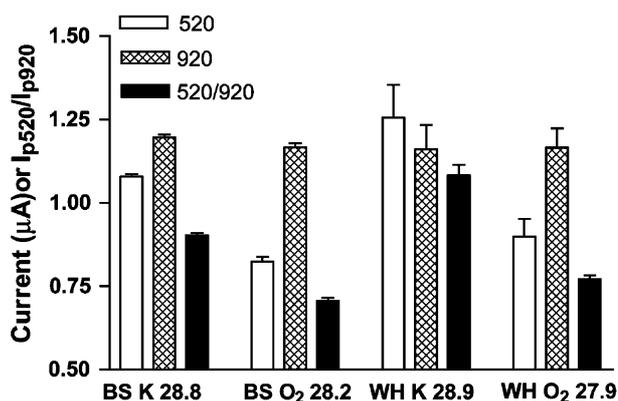
**Figure 4** Voltammetric peak currents measured at 520 and 920 mV and the signal ratios,  $I_{p520}/I_{p920}$ , for similar kappa number pulps.
