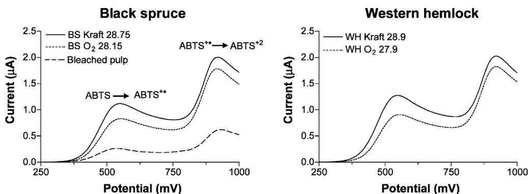
**Figure 3** Voltammograms of ABTS (0.2 mM) in the presence of fully bleached pulp and with kraft and oxygen delignified pulps from black spruce and western hemlock with similar kappa number:  $28.4 \pm 0.5$ .
