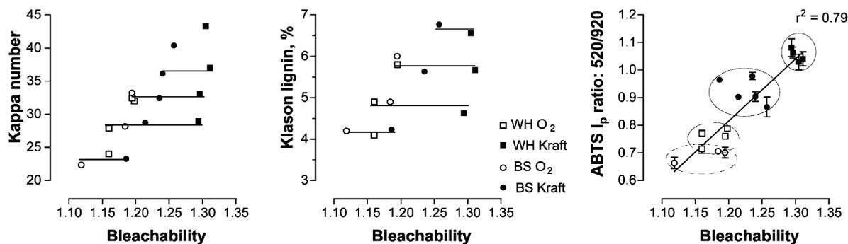
**Figure 5** Variation of the bleachability of D<sub>0</sub>E stages for different types of pulp at various kappa numbers (left) or Klason lignin contents (middle) and relationship between pulp bleachability and voltammetric signal ratio  $I_{p520}/I_{p920}$  of ABTS with the same series of pulps (right).
