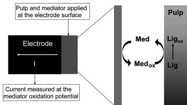
**Figure 1** Cyclic voltammetry of pulp in the presence of mediator to measure the content and reactivity of residual lignin in kraft pulp.
