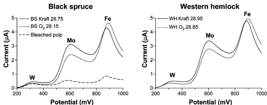
**Figure 7** Voltammograms of equimolar mixture of transition metals mediators (0.5 mM each) with brownstock kraft and O<sub>2</sub>-delignified pulps from black spruce (left) and western hemlock (right). A voltammogram of mediators with fully bleached pulp is also shown (left).
